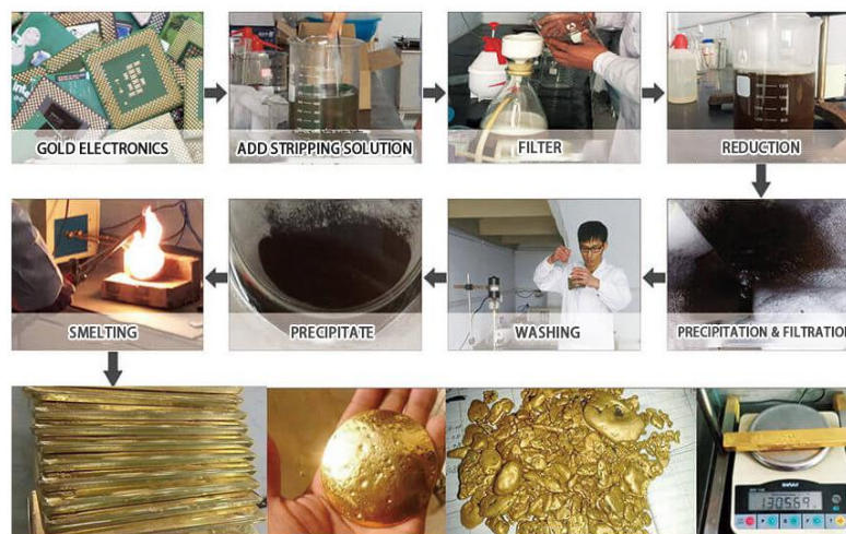
3-18. Figure_ Flow chart precious metal recovery [ https://www.alibaba.com/ ]
