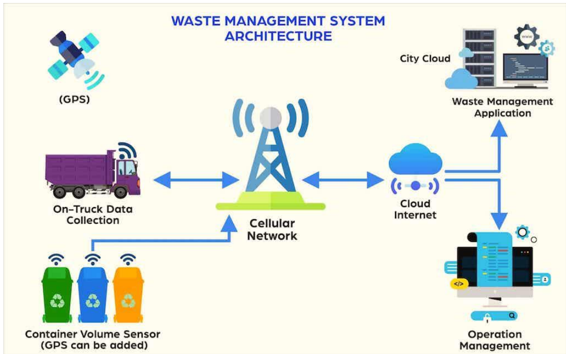
6-1. Figure_Waste Management System Architecture
