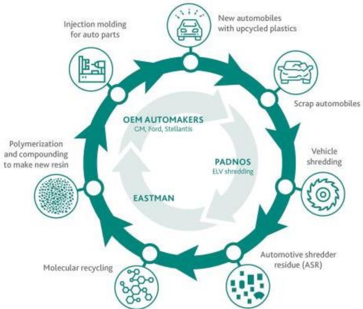
3-3. Figure_Closed-loop recycling of automotive mixed plastic waste
