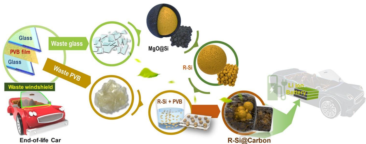
4-4. Figure_Schematic of the synthesis method of reduced silicon and silicon/carbon composites for lithium-ion batteries
